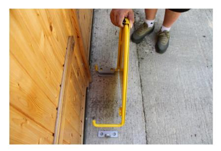
Mark the 4 holes with a pencil on both brackets on the surface.
