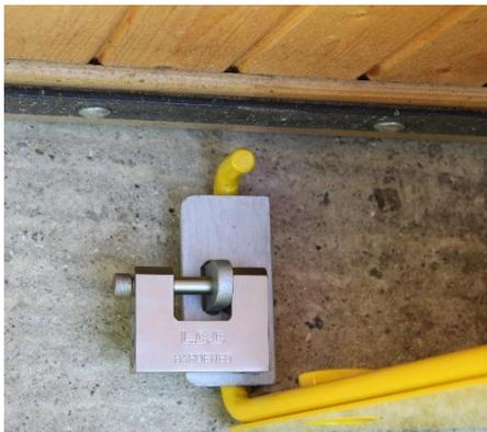
*10. Last of all, lock with padlock to secure the device.*
